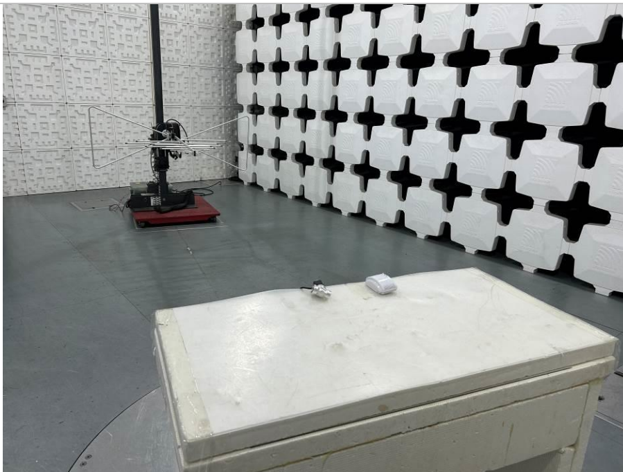
Radiated emission (30 MHz–1000 MHz)
