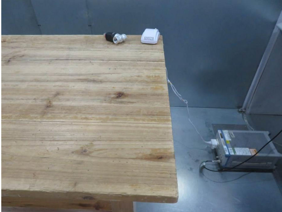
Radiated emission (30 MHz–1000 MHz)
